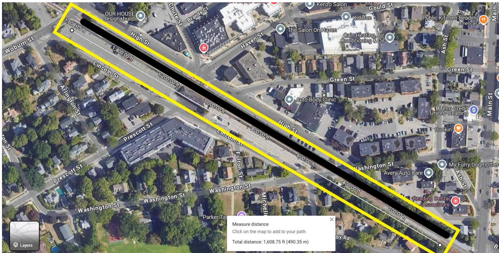
Figure 2: Satellite view showing ~1,600ft of double track between Main Street (Rt. 28) and Woburn Street.
