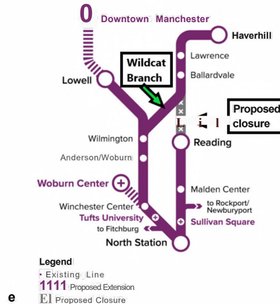
Figure 1: Modified TRANSITMATTERS route map showing the Wildcat Branch (in Wilmington) and the proposed closure of the track between Reading and the Wildcat Branch. TRANSITMATTERS recommends moving the Haverhill Line to the Lowell line via the Wildcat Branch, allowing the closure of track between Reading and Wilmington.
