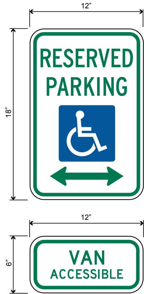
TC-P-ADA-V-RE-MA POLE MOUNTED ADA PARKING REGULATORY SIGN W/ VAN ACCESS (RE-ENGINEERED) SCALE: NTS NOTE: BOLLARD BY G.C.
