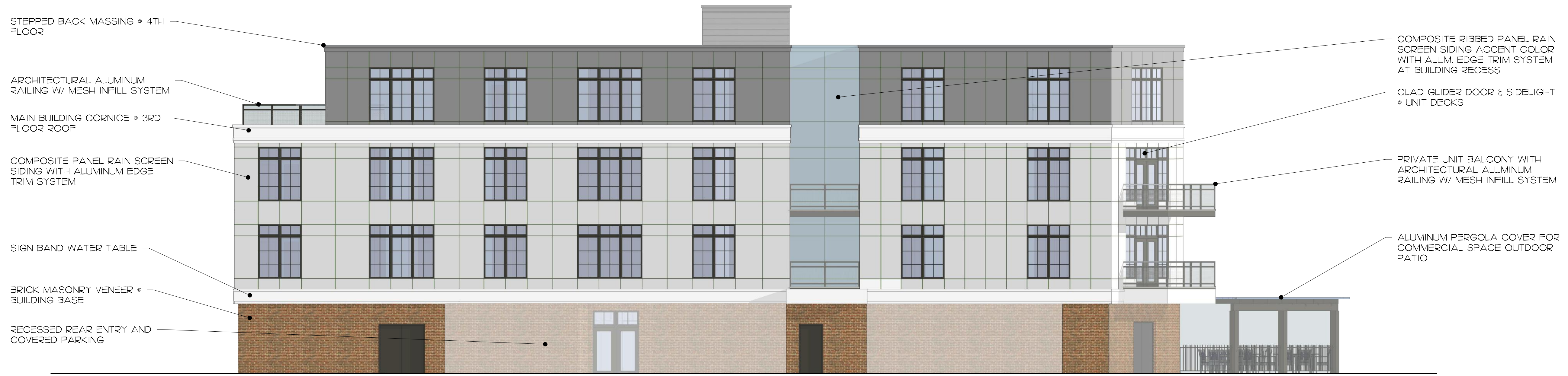
1 FRONT ELEVATION (HAVEN STREET) Scale: 1/8" = 1'
